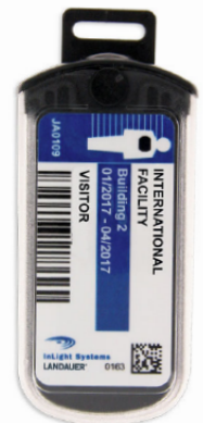
The Neutrak dosimeter can be enclosed inside the InLight holder
