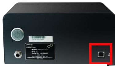
Figure 4-3: Reader USB Connection
