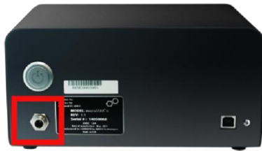
Figure 4-2: Connecting Reader Power
