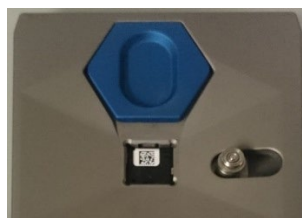
Figure 3-2: Correct nanoDot Orientation
